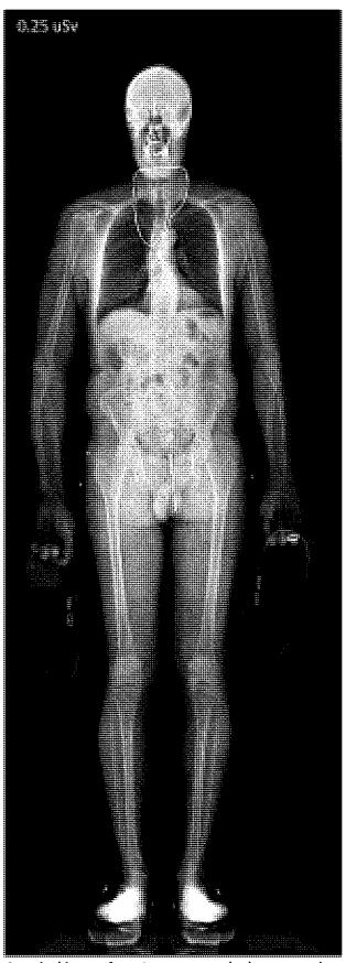
A typical image from Intercept on the lowest setting, 0.25 uSv. Items: teeth fillings, neck chain, object in shoe heal, ring and zipper. Intercept can operate at up to 200 uRem for even better image qually.
